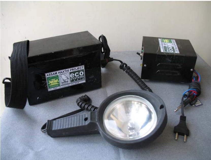
Figure 4. A spotlight for deterring elephants. Made using local materials and ideal for fluctuating electricity supply.
